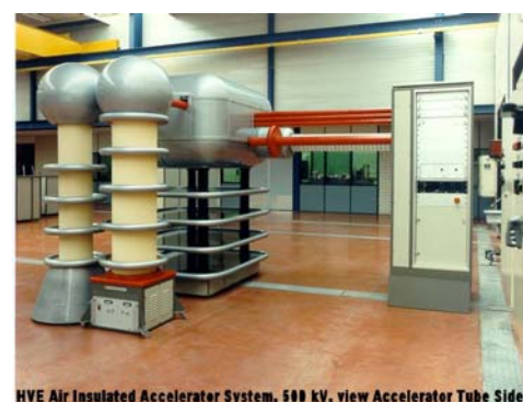
HVE Air Insulated Accelerator System, 500 kV, view Accelerator Tube Side
