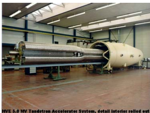
HVE 5.0 MV Tandatron Accelerator System, detail interior rolled out
