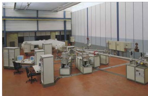
HVE 3.0 MV Tandatron Accelerator System equipped for IL, RBS and PIXE
